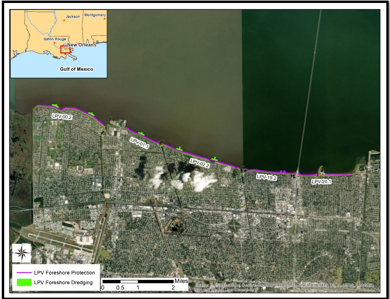
Figure 2. Foreshore protection placement and construction access dredging areas.
